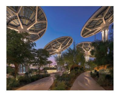
"The fusion of solar power technology with the shading of its striking 'treelike' canopy structures gave clearly defined purpose to all the engineered design elements. Natural outdoor light for a power-generation strategy and shading cleverly reduce energy needs for cooling co-located spaces and additional lighting is reservedly employed only where and when needed, with responsive controls."
